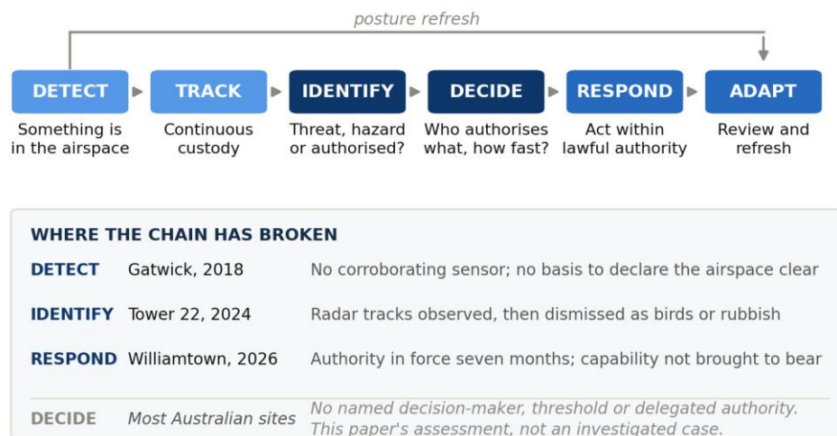
Figure 4: The counter-drone chain, and where the documented failures cluster. Detection is necessary and rarely sufficient; the binding stages sit in the middle. The three named cases are investigated incidents. The decide row beneath the rule is this paper's assessment and is not drawn from an investigation record.
